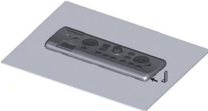
5. Use the tool to raise the panel at the two notches on the upper side of the unit.
