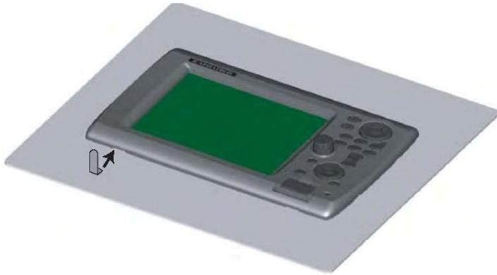
2. Pull the tool to raise the panel slightly. Repeat this action for all notches on the lower side of the unit
