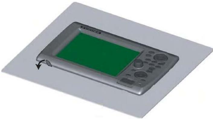
3. Insert the tool into the small notches located on the sides of the panel, and pull the tool to raise the panel slightly
