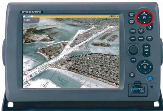
On the MFD8/12, a generic **USB mouse** connected to one of the **USB ports** is **required** to perform the initial configuration.
